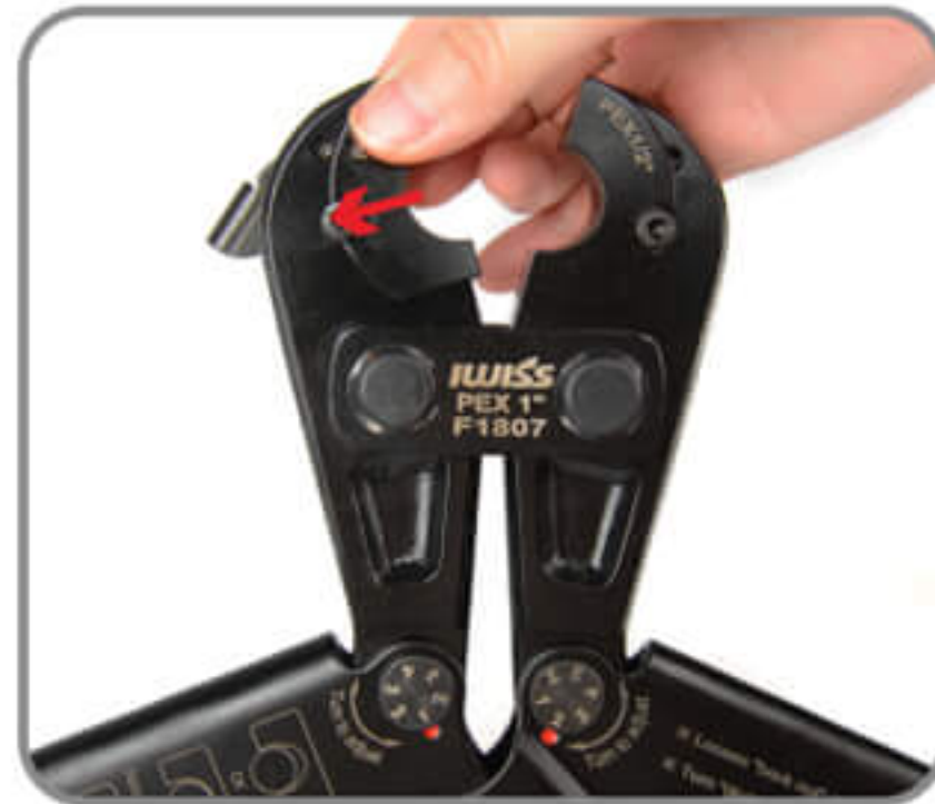
5. Lift up the fixing pin and push into the press jaw
