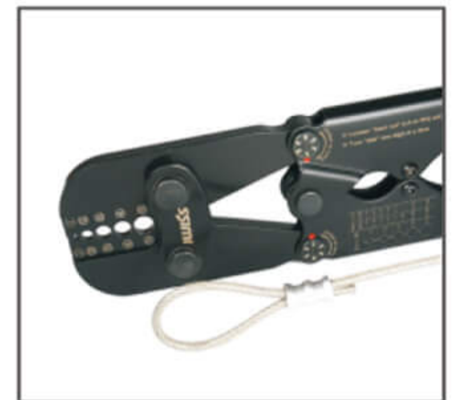
4. Close the crimp tool to make an eye splice on the wire rope.
