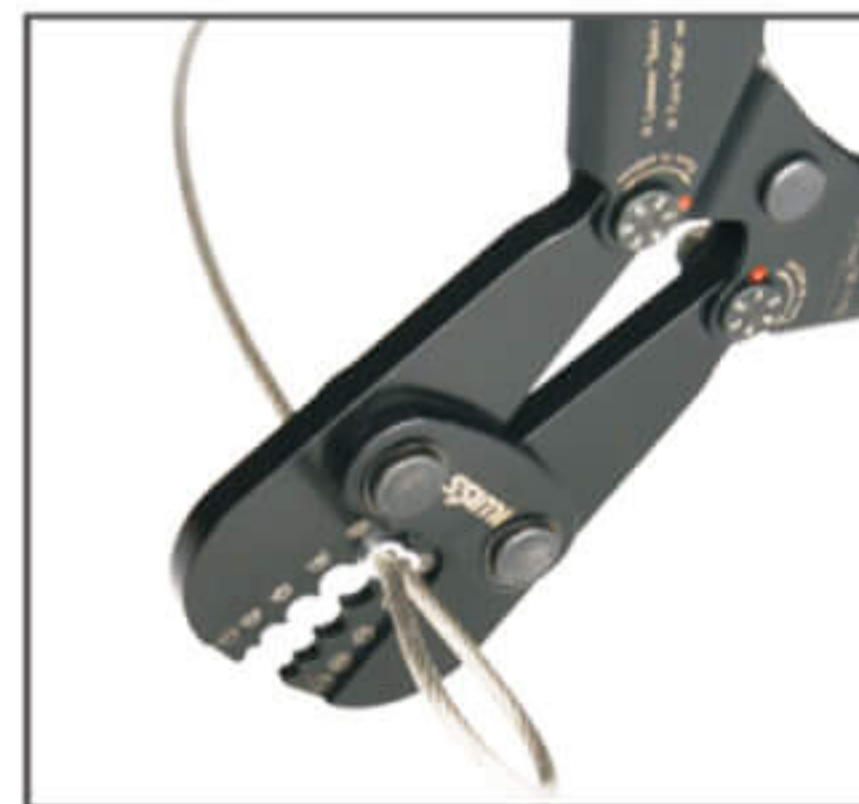
3. Place the sleeve into correct slot size of the swager, and make sure the sleeve is positioned upright in the swager slot.
