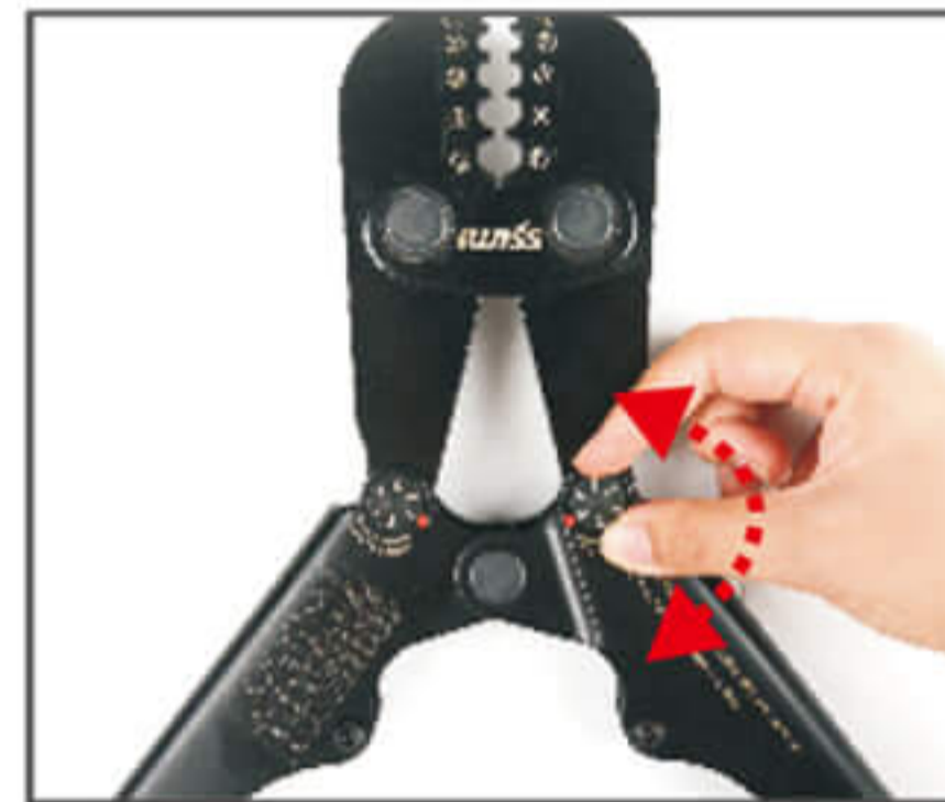
3. Calibrate the swager by dialing the two Strength Control Buttons clockwise or anticlockwise.
