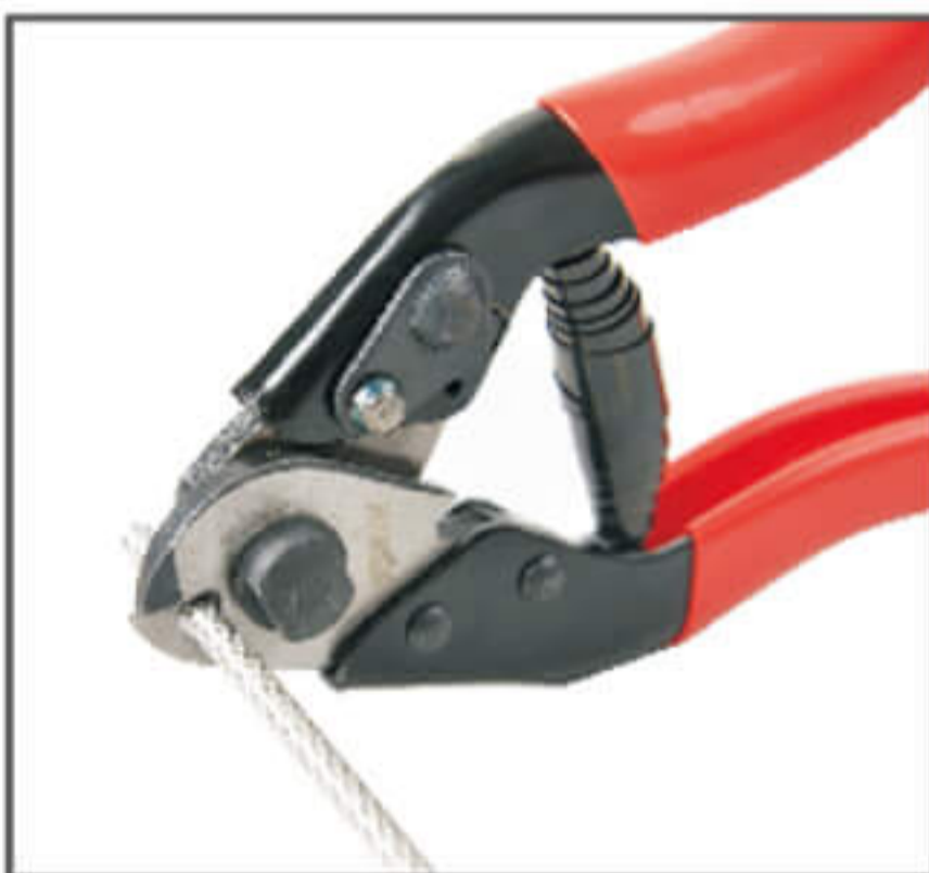
1. Cut off certain length monofilament or strand cable with IWS-7 cutter, thread the sleeve onto the leader line.
